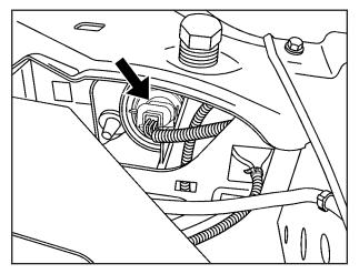
3. Turn the bulb socket counterclockwise to remove it from the headlamp assembly.
